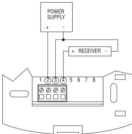
Figure 3: Voltage Output
