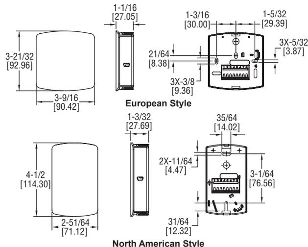
The **Series BTT-E/N Wall Mount Temperature Transmitter** is used to monitor the temperature in a room or indoor building space and transmit the measurement to a remote display, building management system, or control system. The transmitter signal output offers more reliable signal accuracy over long wire runs when compared to standard thermistor or RTD sensors.
