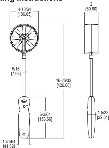
The **Model VP2 Wireless 100 mm Vane Thermo-Anemometer Probe** measures air velocity, air flow, humidity, and temperature when combined with Models UHH and UHH2 or the Dwyer Mobile Meter app. By having a larger diameter, the rotating vane is able to measure velocities down to 50 fpm or 0.25 m/s. An arrow is molded into the vane housing to depict the flow direction.
