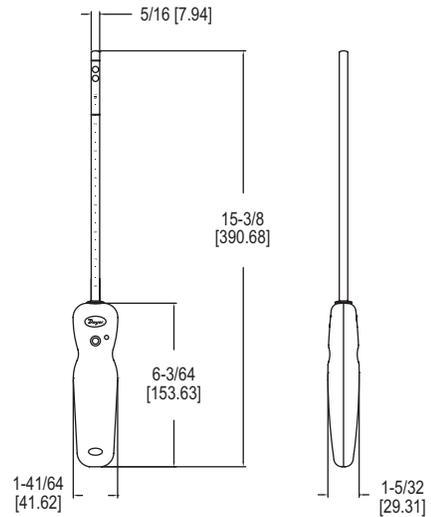
The **Series AP2 Wireless Thermo-Anemometer Probe** measures air velocity, air flow, and temperature when combined with Models UHH and UHH2 or the Dwyer Mobile Meter® app. In order to prevent damage to the sensing element, the probe has a protective sleeve that slides over the sensor when it is not in use. Markings on the probe allow users to know the insertion depth to obtain better accuracy when traversing the duct.
