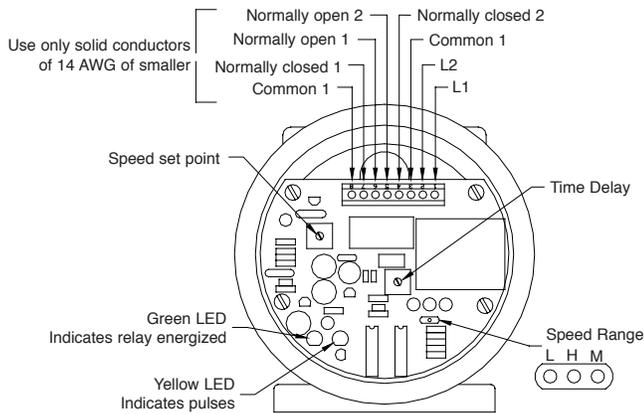
Remove end cap to expose terminals and pick-up speed adjustment screw. Wire input power from source to terminals L1 & L2. Be certain to use the provided ground screw. The output of the Series DSS is a DPDT relay. There are two sets of output contacts. Each set includes normally open, normally closed and common. As a result, the unit can be used to control two separate circuits such as a motor starter and a signal light.
