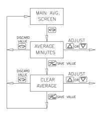
Press the SETUP key from the MAIN AVERAGE screen to enter the AVERAGE setup screen. Use the UP/DOWN arrow keys to adjust settings to the desired values. Press the ENTER key to save a value and proceed to next setup screen. Press the SETUP/ESCAPE key to return to the main average screen without saving the current parameter's value.
