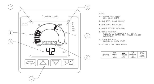
The control unit has two alarm relays which are individually activated when the reading continuously exceeds the alarm setpoint for the amount of time delay specified. Each is an SPST (FORM A) relay contact output.
