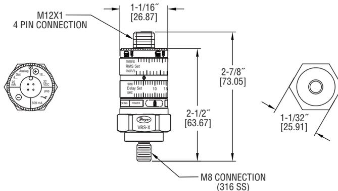
The Series VBS Vibration Switch is small, compact, and uses two easy set up dials that adjust the maximum RMS velocity set point and false trip time delay. The Series VBS is intended to continuously monitor the changes in a machine's vibration level. The VBS takes real-time RMS vibration input and provides an analog output of velocity, as well as a switching output when an alarm value is exceeded.
