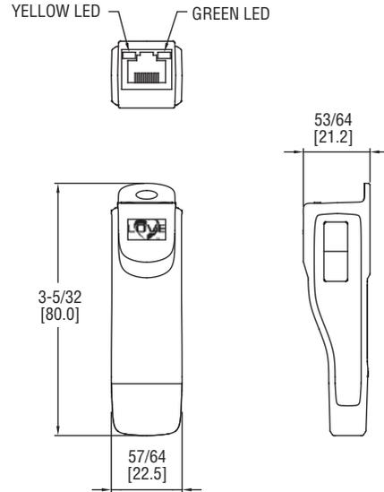
The Model MN-1 Mini-Node Communication Signal Converter is a low cost device that converts half duplex RS 485 serial communications signals into a signal that can be read by any computer with a USB port. The integral USB connector and RJ-45 connector reduces set up time by eliminating extra wiring. The Model MN-1 is powered via the USB connection which eliminates the need for an external power source. The compact size is great for field installation, control panels, and lab testing.
