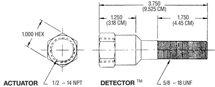
**Series DT Detector position sensors** consist of two basic components, a hermetically sealed reed switch sensor assembly and a magnetic actuator assembly. A change in state of the contacts in the sensor is initiated by moving the actuator closer to or further away from the sensor target area, either into or away from the reed switch magnetic sensing range. This opens or closes the electrical circuit.
