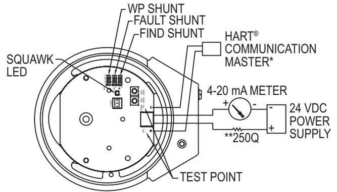
\*OPTIONAL, MAYBE CONNECTED TO TEST POINT AS SHOWN OR TO SCREW TERMINALS
