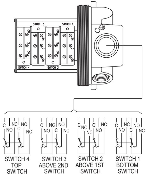
**Figure 4: Wiring for switch type D. 1, 2, or 4 switches**
