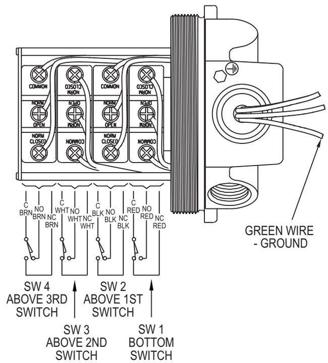
**Figure 3: Wiring for factory sealed leads option. 1, 2, or 4 switches. Switch 1 wires are red, switch 2 wires are black, switch 3 wires are white, and switch 4 wires are brown. Wires are labeled C, NO, NC**
