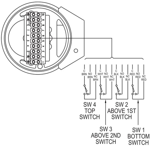
**Figure 6: Wiring for switch types C, R, V and W. 1, 2, or 4 switches**
