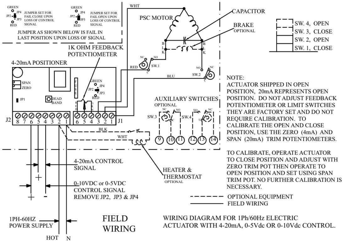
**Electric Actuators Wiring Diagram: ACT-TD & ACT-MD**
