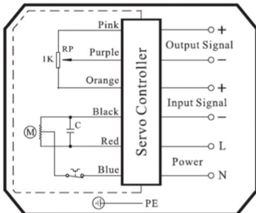
**Note:** To speed up installation of the control wires to the ACT-MDXX modulating actuator, it is recommended to remove the control module from the actuator. The control module can be removed by removing the two mounting screws on the left and right of the control module. Install the control wires to the correct terminal points and then reinstall the control module.
