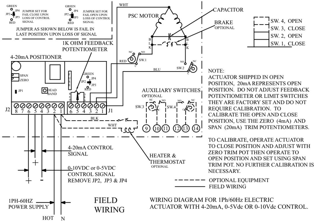
Electric Actuators Wiring Diagram: ACT-TD & ACT-MD
