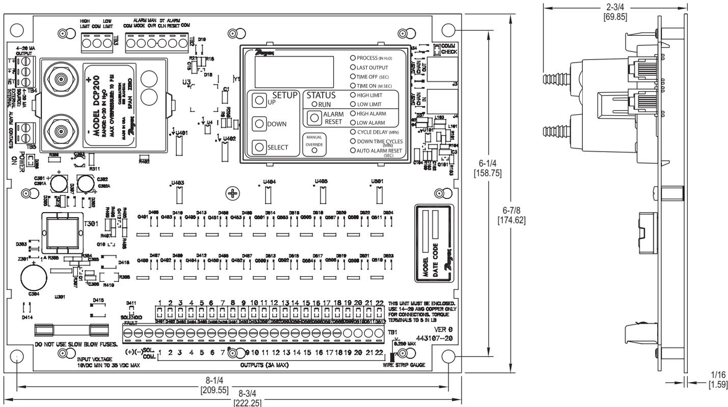
Figure 1 – Dimensional Specifications for the DCT100DC (shown with optional module DCP100A)
