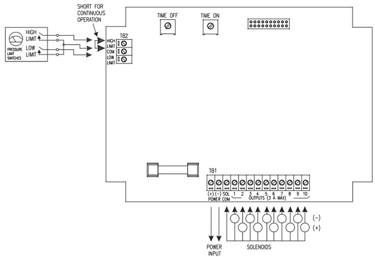
Figure 2-2 Wiring Connections DCT604, DCT606, DCT610
