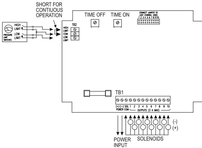
Figure 2-1 Switch Connections
