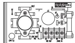
The Series BPS Building Automation Power Supply is used to convert 24 VAC to a regulated DC power source for transmitters with 4 to 20 mA outputs. The output voltage can be field adjusted from 1.5V to 27V using a potentiometer. The 3A fuse protects the power supply from over-current conditions. The snap-on bracket can be quickly surface mounted to any flat surface.
