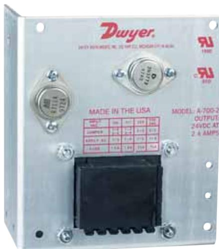
The **Model A-700** economical and reliable power supply is suitable for powering all Dwyer<sup>®</sup> pressure, temperature or air velocity transmitters. Inexpensive, open-frame design allows convenient access to input/output solder terminals. Auxiliary inputs are selectable for operation from power sources found worldwide. Compact size eases enclosure installation. UL and CSA approved.
