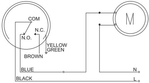
**Figure 10-Double Function (Filling (NC))**
