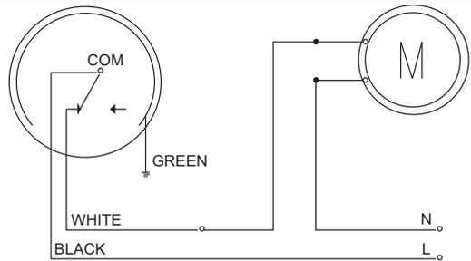
**Figure 12-Filling (NC) Function**
