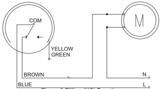
**Figure 8-Filling (NC) Function**
