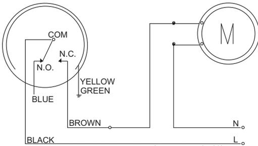
**Figure 9-Double Function (Emptying (NO))**
