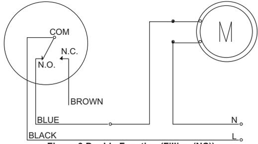
**Figure 6-Double Function (Filling (NC))**
