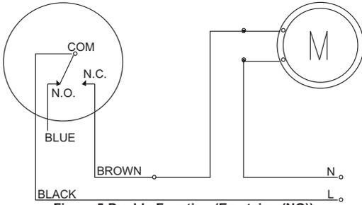
**Figure 5-Double Function (Emptying (NO))**
