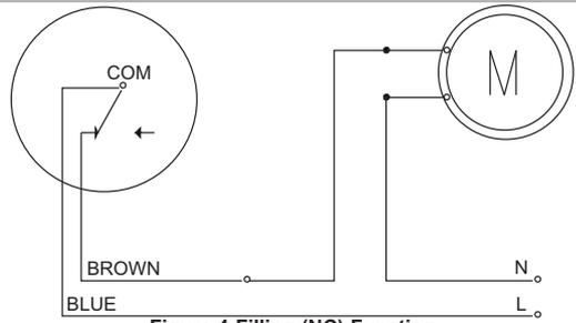
**Figure 4-Filling (NC) Function**
