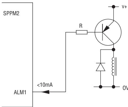
Figure 4: Driving a Relay using Alarm Output
