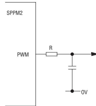
Figure 6: Using PWM Output to Convert Digital to Analog
