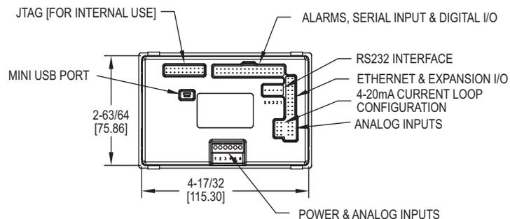
The **SERIES SPPM2** Graphical User Interface Panel Meter is a configurable, full-color 4.3" (109 mm) touch screen display that can be used in a variety of applications. By using the free Windows® based Interface Panel Design Studio software, users can personalize the display to suit their needs. A development kit is also available, which a development board with buttons, dials, LEDs, and screw terminals to test the functionality of all inputs and outputs.
