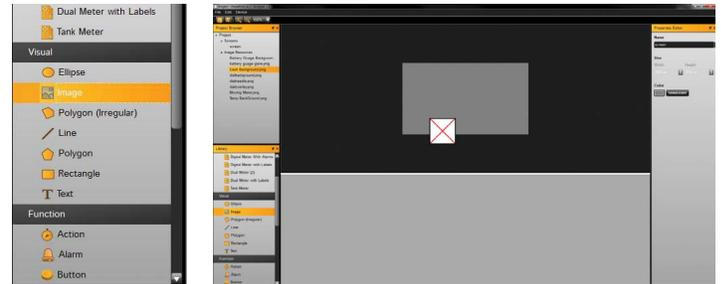
10. To add the meters: a) Add in meter images in the same way as mentioned in step 9. b) To resize the images, grab the corners or sides and stretch them to the necessary size. c) Once finished, click on the individual meters and name them for easy access later.
