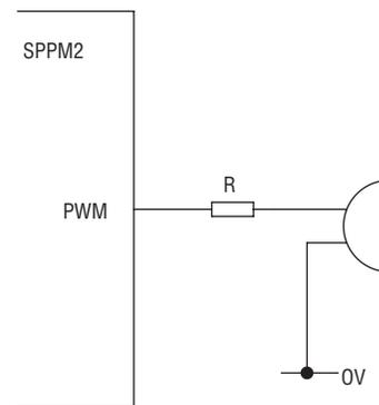
Figure 7: Using PWM Output to Drive a Buzzer
