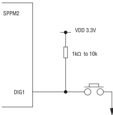
Figure 5: Generating a Digital Input with a Push Button
