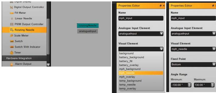
16. To test the app, click File>Preview or press F5 to bring up the simulation window. Inputs can be simulated in this screen to verify that everything is working properly.
