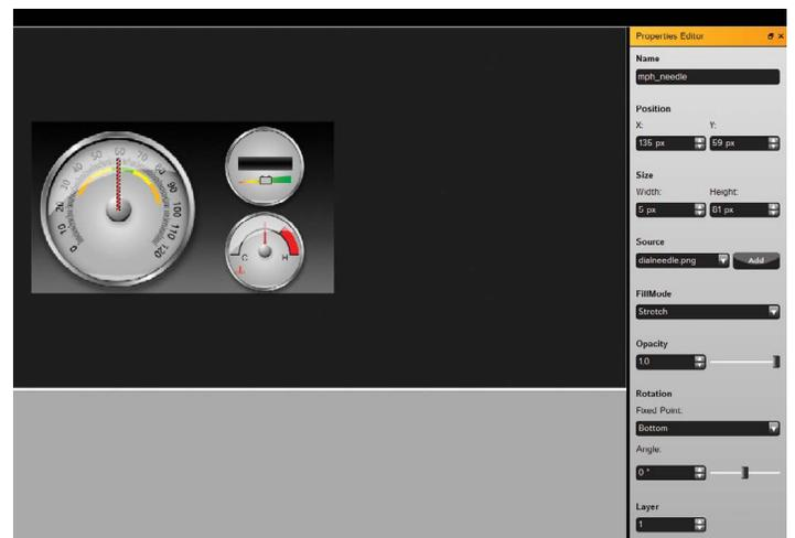
12. To add the battery gauge: a) Add the gauge photo as mentioned in step 9. b) Drop the image into position and name it.
