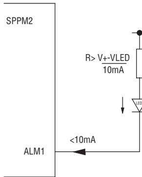
Figure 3: Driving an LED using Alarm Output
