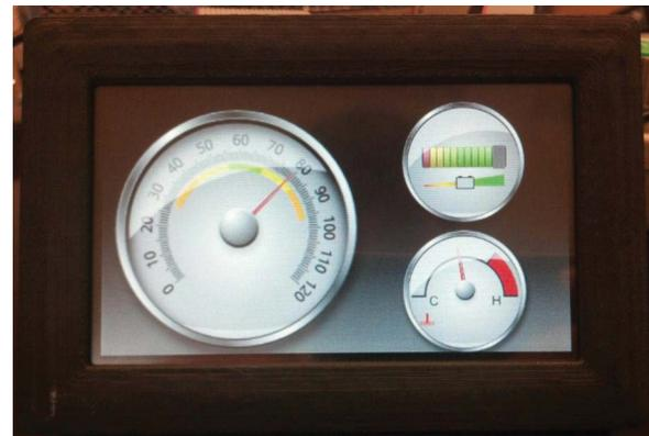
14. Click on analogueInput and assign the wanted channel to control the mph\_needle. Here, also set the voltage range and what value that voltage range translates to on the display. Follow the same instructions to add any other needle channels.
