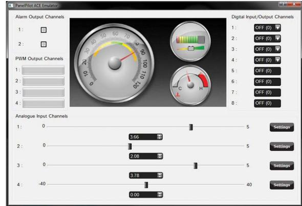
17. Once satisfied with the simulation, click File>Upload or press F6 with the meter still plugged in to send the app to the display.
