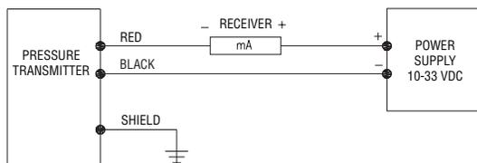
The maximum receiver load resistance ( $RL_{max}$ ) for the DC power supply voltage ( $V_{sup}$ ) is expressed by the formula:
