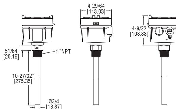
The Model VRLS Vibrating Rod Level Switch is an economical choice in level detection of powders and bulk solids. Ideal for silo or hopper applications, its probe design allows for self-cleaning, ensuring no build-up of material and accurate detection. Sensitivity is adjustable for detection ranging from large granular material to small powders with low bulk densities.
