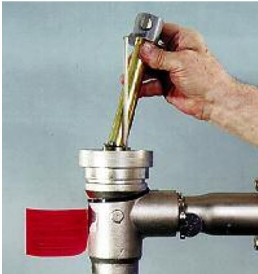
4. Seat the O-ring on the sight tube, lubricating it with a small amount of service-compatible silicone grease or petroleum jelly to facilitate replacement.
