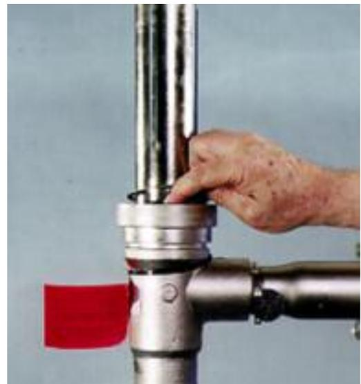
If reassembled correctly, the center of the ball indicator should lineup with the scale “zero” (either dotted black or scribed line). If it does not, disassemble the meter completely and carefully reassemble it, making sure the slotted meter tube is completely seated in the body.
