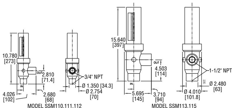
**Series SSM 31 All Metal Flowmeters** are ideal for dirty or opaque fluids, high temperature and high pressure service and harsh environments. The direct reading scale provides  $\pm 2\%$  accuracy. Flowmeters can quickly be disassembled without removing the body from the pipeline for easy cleaning.
