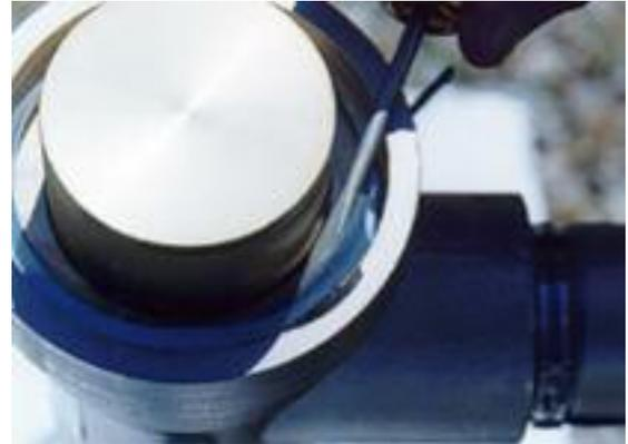
3. Using hands only, pull the sight tube straight up out of the body with a slight twisting motion, lifting it clear of the body and snorkel. The inner flange ring will lift off with the sight tube.
