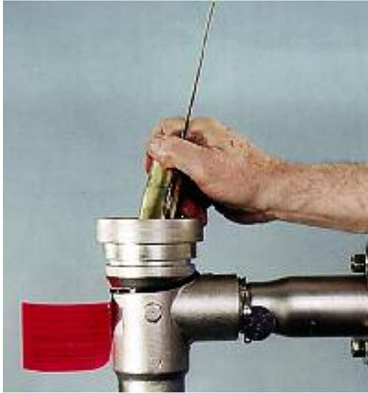
2. Place the spider over the meter tube with the “notched leg over the snorkel tube or guide rod. Slide the spider down to the meter tube’s shoulder.
