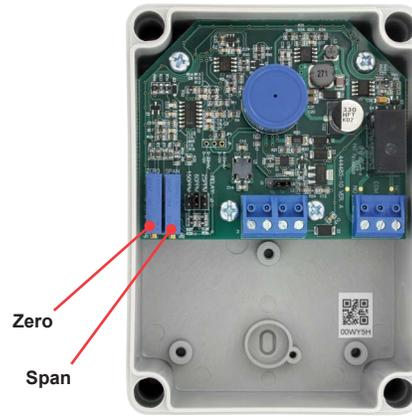
Figure 6: Calibration controls
