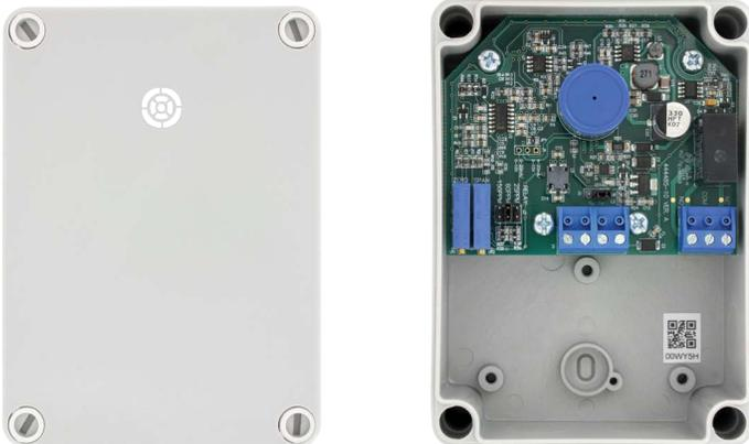
Figure 5: Circuit board mounting screws
