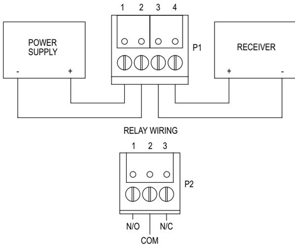
Figure 2: Current and voltage output and relay wiring
