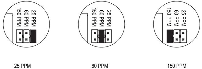
Figure 4: Relay jumper positions
