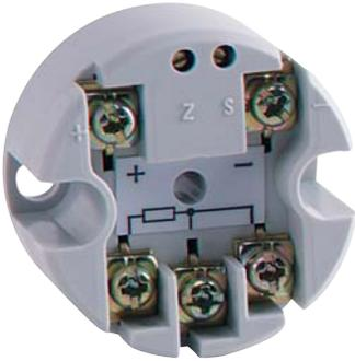
The device is a low cost temperature transmitter designed to accept a standard platinum resistance sensor (Pt100 2 or 3 wire) to BS1904 or DIN 43760 and convert the temperature to an industrial 4-20mA current. It is housed in a DIN standard connecting block.
