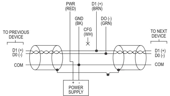
Figure 3: BACnet individual power supply wiring
