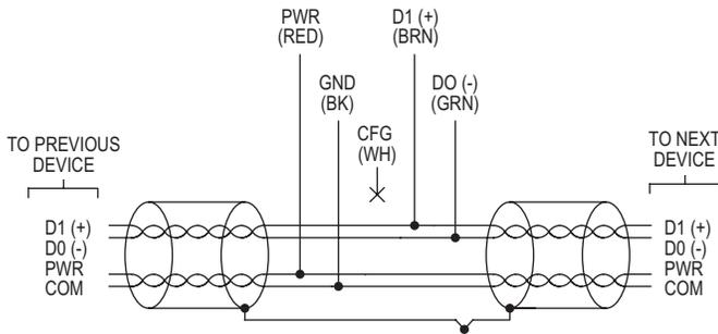
Figure 2: BACnet common power supply wiring
