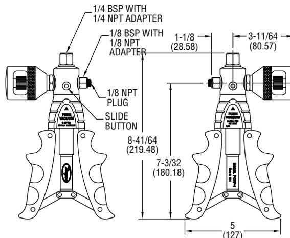
The Series PCHP Pneumatic Hand Pump comfortably sources pressure and vacuum to check calibration of gages, switches, transmitters, and recorders. The contoured cushion handles provide extra comfort while preventing the pump from sliding. The oversized check valve provides smooth operation throughout the output range. The dual o-rings on all pistons ensure zero leakage.
