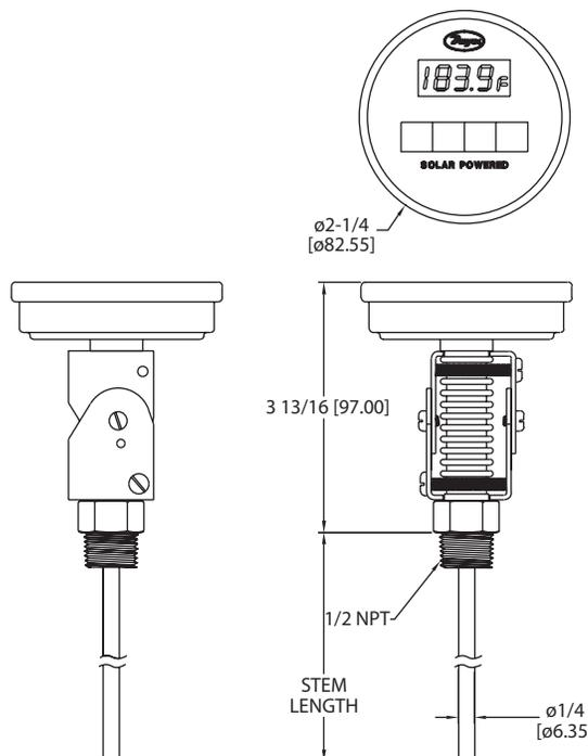
The Series DBT Digital Solar-Powered Bimetal Thermometer takes the guesswork out of temperature measurement. The 3-1/2 digit LED display is easy to read and provides resolution to 0.1°F. The adjustable angle can be mounted in virtually any position. The engineering units can be selected in the field by removing the back cover.
