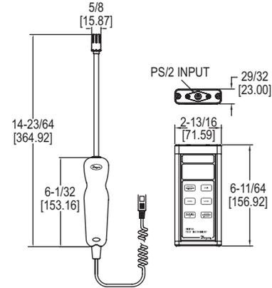
The **Model 485B Thermo-Hygrometer** is a versatile, compact, handheld instrument for measuring percentage of relative humidity and temperature in °F or °C. Dew point and wet bulb temperatures are derived from the relative humidity and temperature measurements and are displayed on the LCD.
