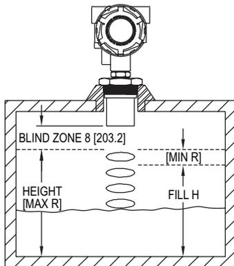
Figure 8: Target calibration
