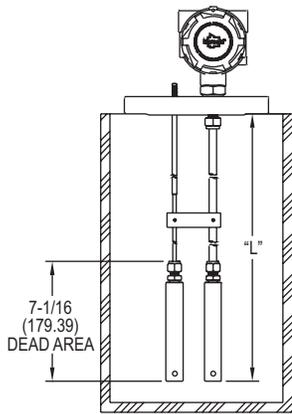
Figure 1: Attached Ground Rod Option
