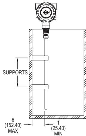
Figure 2: Supports to Tank Side Wall
