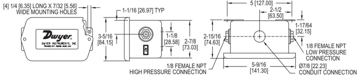
Monitor differential pressure in air/liquid flow systems, HVAC automation, pneumatic systems and process control with the **Series 647 Wet/Wet Differential Pressure Transmitter**. Units are temperature compensated and provide a 4-20 mA output signal which can be interfaced with chart recorders, data loggers and computerized monitoring and control systems.
