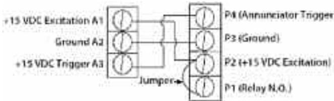
below, the remote annunciator connector is at left, and the RSM connector is at right: Connect P1 to P2, then connect P2 to A1 (Located on Remote Annunciator), finally connect P3 to A2 and P4 to A3.
