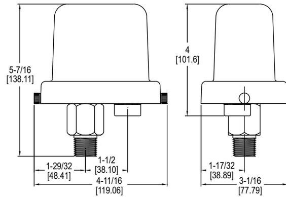
The **Series A1F Compact OEM Pressure Switch** is ideal for panel mounting wherever a high-quality, economical open-case or weatherproof control is required.
