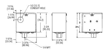
The Series CS Low Cost Diaphragm Pressure Switch is ideal for instrument panels, small compressors and general industrial applications. Visible set point and easy-to-wire SPDT snap switch reduce installation time. This switch operates in any position and is vibration resistant.
