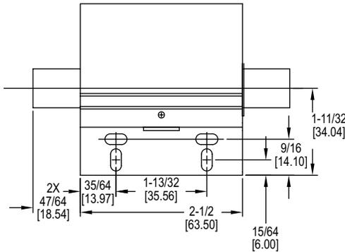
Figure 2: Mounting Hole Dimensions
