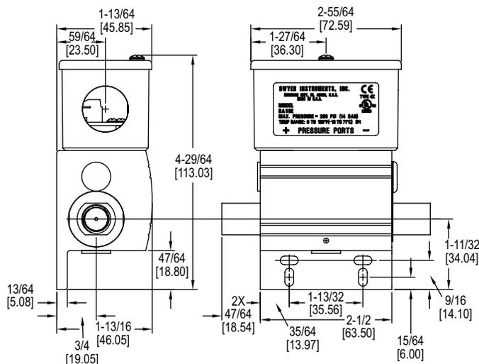
The **SERIES DX** is a pressure switch that makes a contact output based on the differential pressure between two pressure sources. Unit incorporates a SPDT snap switch in a weatherproof, type 4X enclosure. Series DX features low differential pressure set points with high single pressure limit.
