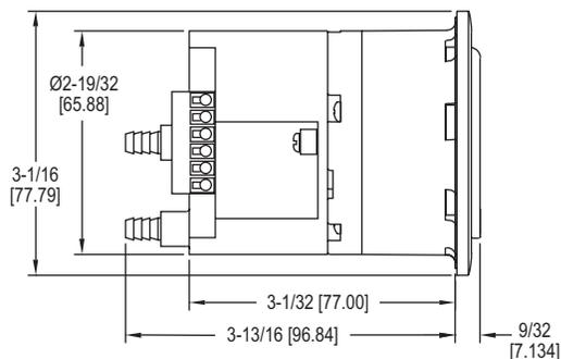
The **Series MP Mini-Photohelic® Differential Pressure Switch/Gage** combines the time proven Minihelic® II differential pressure gage with two SPDT switching setpoints. The Mini-Photohelic® is designed to measure and control positive, negative, or differential pressures consisting of non-combustible and non-corrosive gases. Gage reading is independent of switch operation. Switching status is visible by LED indicators located on the front and rear of the gage.
