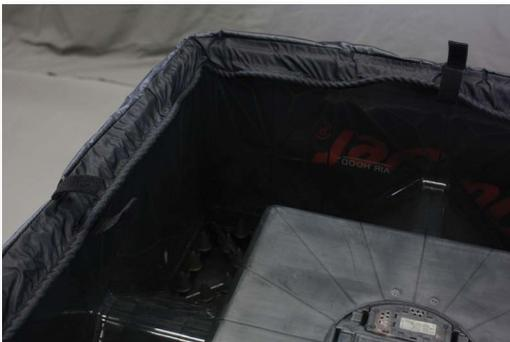
5. Place the lower 2' x 2' adapter frame into the SAH over the top of the inner cord loop skirt trapping the cord inside the SAH and loosely close the hook and loop straps over the adapter frame to hold it in place.
