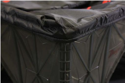
4. Fold the canvas hood inside out over the SAH, exposing the inner cord loop and place that cord loop inside the SAH unit. Pay special attention to the corners. Open the fabric hook and loop straps if they are closed.
