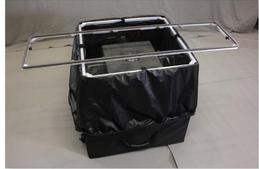
6. Assemble the required upper frame system that matches the adapter hood choice. Details for which pieces are needed for each hood size are on page 2. Starting with two pieces that fit together, loosen the knob on the first piece. Slide the second piece so the grooves fit around the knob on the first piece. Tighten the knob to hold in place. Continue until entire upper frame is assembled.
