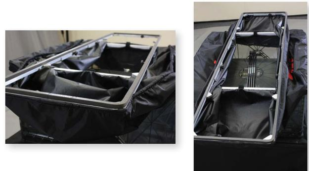
8. Stretch the top cord loop of the canvas hood onto the upper frame, aligning the corners of the frame with the sewn seams of the canvas hood. Once they are aligned, press the cord into the groove all the way around the frame.
