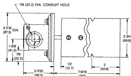
The Model 530 Air Flow Switch provides excellent sensitivity and reliability at a very reasonable price. Quality features include rugged die cast zinc body, stainless steel vane, silicone rubber gasket and SPDT snap switch. Unit is easily field adjustable from 400-1600 FPM. Mounting is fast and simple, requiring only two screws. Vane fits 6 in. or larger ducts. UL approved. To order, specify Dwyer Instruments, Inc. Model 530 Air Flow Switch.
