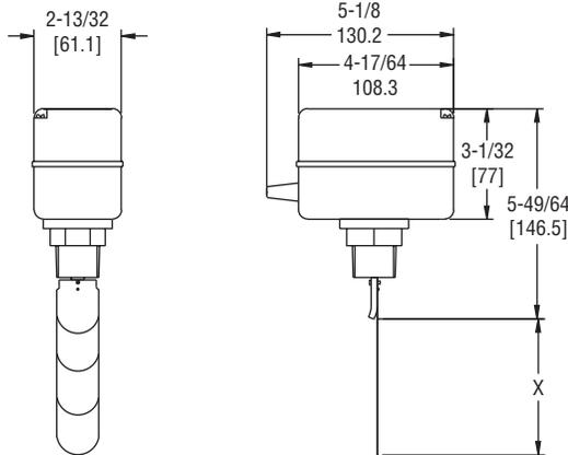
The **Model FS-2 Paddle Flow Switch** offers an economical flow proving solution. Custom set points tailored for the application are enabled by field adjustable vane layers and a set point adjustment screw. The FS-2 features an aluminum weatherproof housing for outdoor installation. Paddles are adjustable to fit 1" to 8" size pipe. FS-2 is ideal for use in "flow or no flow" applications in cold and hot water systems.
