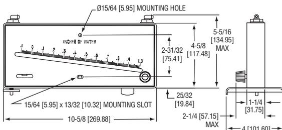
**Dwyer Mark II - Model 40 Molded Plastic Manometers** are ideally suited for air velocity and air filter gage applications at minimal cost. These inclined manometers provide linear calibration and excellent resolution throughout their ranges. They are capable of pressure measurements above and below atmospheric, as well as differential pressure measurements.
