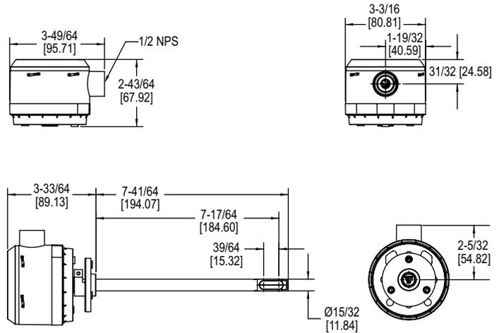
The **Series AVUL Air Velocity Transmitter** quickly and accurately measures air velocity or volumetric flow in imperial or metric units. Simultaneous current and voltage outputs on all models provide universal inputs to monitoring equipment while the output range, units, and 0-5/10 VDC output can be configured via local DIP switches. The optional integral display, or the portable remote display tool, provide a convenient way to locally monitor process values and configure the unit.
