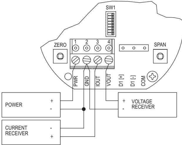
Figure 3: Simultaneous current and voltage output wiring
