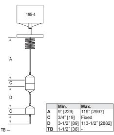
Series 195-6 - Two Stage - Adjustable Differential Each Stage High trip point for lower stage common with low trip point for upper stage
