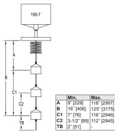
Series 195-8 - Two Stage - Adjustable Differential Each Stage Common trip point at HIGH level
