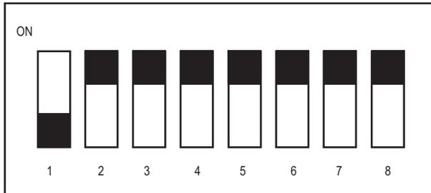
Figure 6: Address of transmitter is 127
