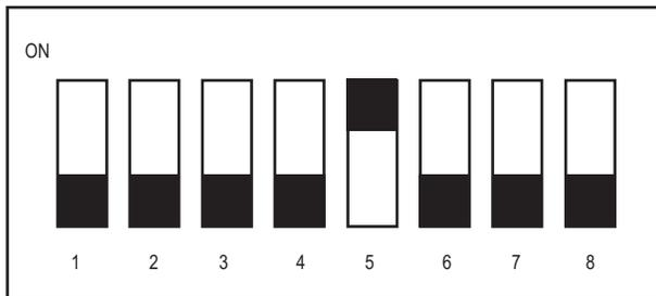
Figure 7: Address of transmitter is 008
