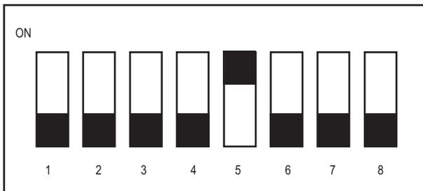
**Figure 7: Address of transmitter is 008**
