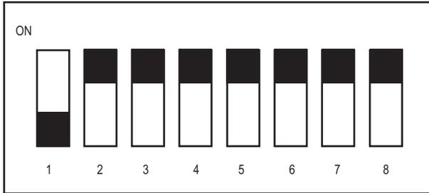
**Figure 6: Address of transmitter is 127**
