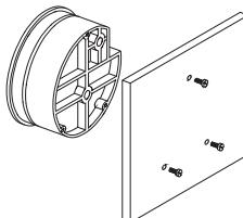
Locate mounting holes, 120° apart on a 4-1/8" dia. circle. Use No. 6-32 machine screws of appropriate length.
