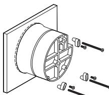
Provide a 4-9/16" opening in panel. Insert gage and secure with supplied mounting hardware.
