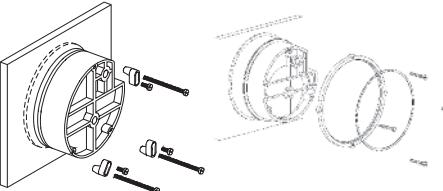
Provide a 4-9/16" dia. (116 mm) opening in panel. Provide a 4-3/4" dia. (120 mm) opening for MP and HP models. Insert gage and secure in place with No. 6-32 machine screws of appropriate length, with adapters, firmly secured in place.
