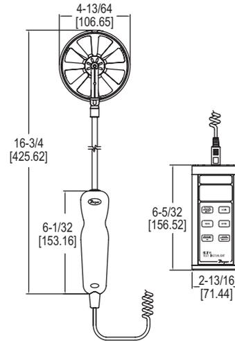
The **Model 473B 100 mm Vane Thermo-Anemometer Test Instrument** is a versatile unit that quickly and easily measures air velocity or volumetric air flow, as well as air temperature and humidity in imperial or metric units. A stainless steel 100 mm vane probe is included, which has a comfortable hand grip. The extruded aluminum housing fully protects electronics, yet is lightweight and comfortable to hold.
