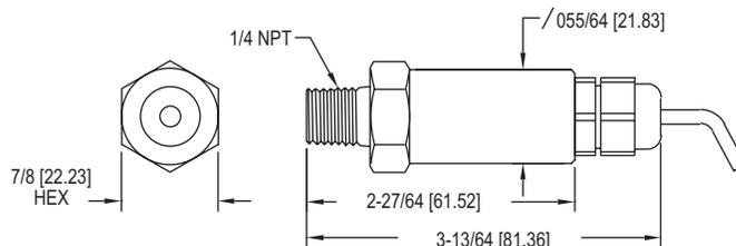
The **Series 626 & 628 Pressure Transmitters** converts a single positive pressure into a standard 4 to 20 mA output signal. The Series 626 and 628 can be used to accurately measure compatible gases and liquids; Series 626 full scale accuracy is 0.25%; Series 628 full scale accuracy is 1.0% (see specifications). Designed for industrial environments with a NEMA 4X (IP66) housing, this transmitter resists most effects of shock and vibration.
